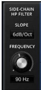
The **Side-chain High-Pass Filter** section allows control over the compressor's sensitivity to low frequencies. That is, the compression threshold becomes frequency dependent and thus less responsive to low frequency content. Three different high pass filter slopes are supported:
