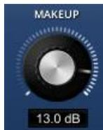
**Make-up gain** is used to compensate the gain-reduction introduced by the compressor. The makeup control can also attenuate the compressed signal up to 60dB which is useful for parallel compression techniques.
