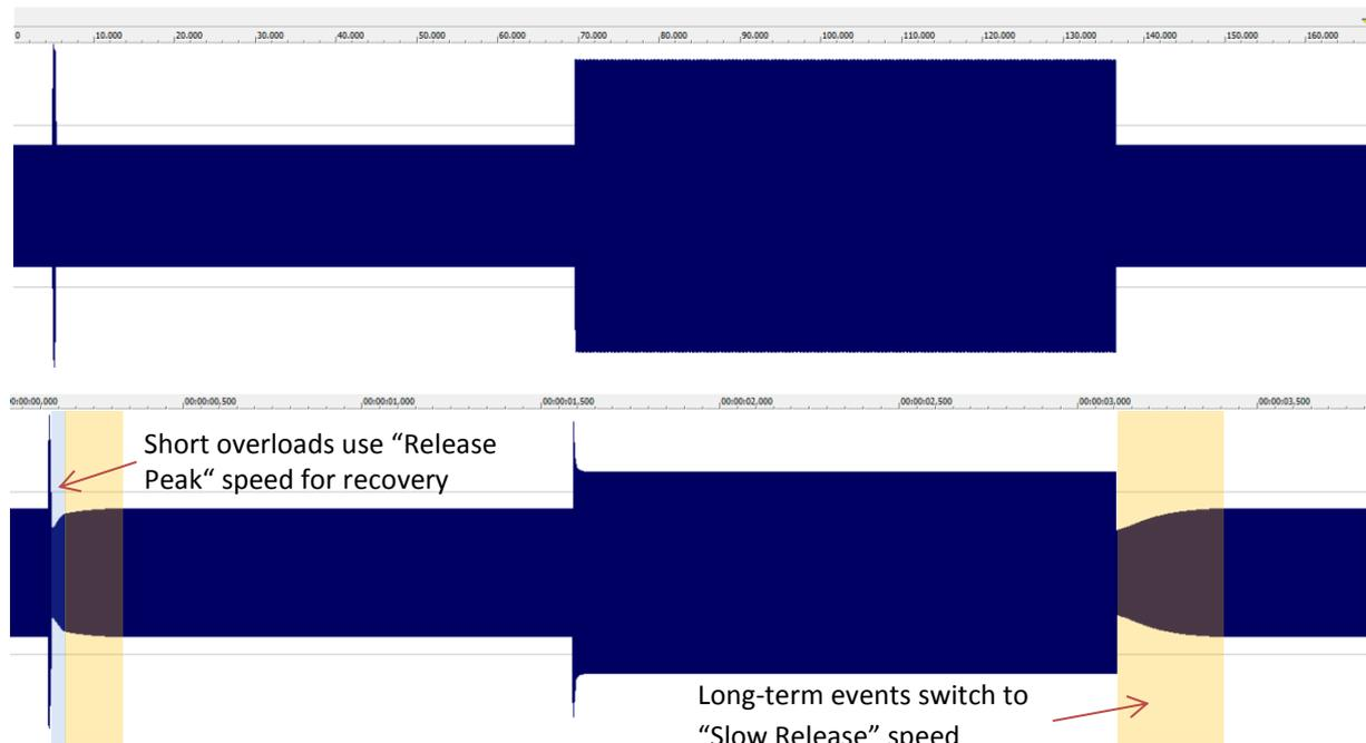
Dual release paths offer a wide range of musically-useful options. For example, single drum peaks can be allowed to recover quickly to avoid “dulling” and “breathing” side-effects. At the same time, sustained content like bass-lines or synth pads can recover slower and thus strongly reduce typical side-effects like “pumping” and distortion.
