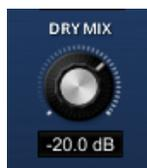
**Dry Mix** blends the original signal into the processed (i.e. compressed) part. It enables the use of parallel compression techniques (upward compression, “NY compression”) without complicated routings or DAW latency compensation issues.
