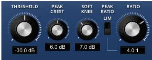
**Threshold** defines the level above which the compressor begins to compress the signal. The lower the threshold, the deeper the “grab” and the more compression.
