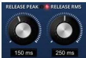
The timing section differs slightly from the typical layout found on most compressors. The TDR Feedback Compressor can dynamically select the most suitable release “path” depending on the program material. Two virtual LEDs indicate the currently active release path and controls.
