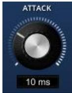
The Attack time controls how long the compressor takes to reach full gain reduction. Fast attack times respond quickly to level changes in the sidechain. Slow attack times on the other hand respond more slowly and smoothly, letting small events (transients) pass through the compressor without gain reduction.
