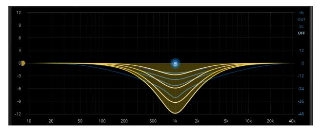
The Q value is the same as before but the threshold curve becomes narrower as threshold deepens. The dynamic EQ curve maintains its constant Q property.
