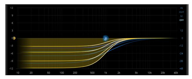
The surgical curve mode is very useful for precise operations such as deep de-essing, the neighbor frequencies are much less affected. The main drawback is a greater CPU load.
