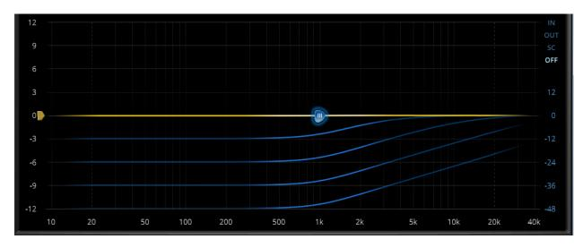
Peaking filters' Q for threshold decreases with gain ("inverse proportional Q behavior"). For shelving filters, we see the corner frequency seemingly being shifted in dependence of gain.
