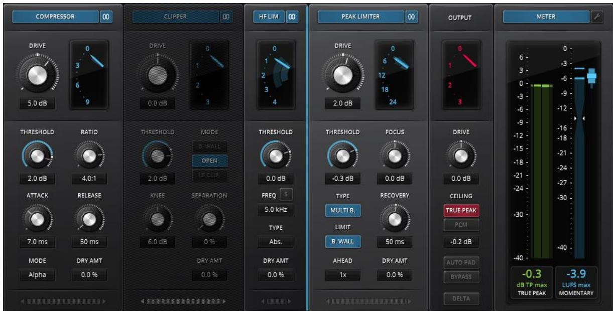
The four primary processing modules can be reordered to taste. Simply drag the module at the handle and drop it wherever needed (the handle can be found at the bottom of each movable module). Alternatively, clicking either arrow will move the given module one step left or right.
