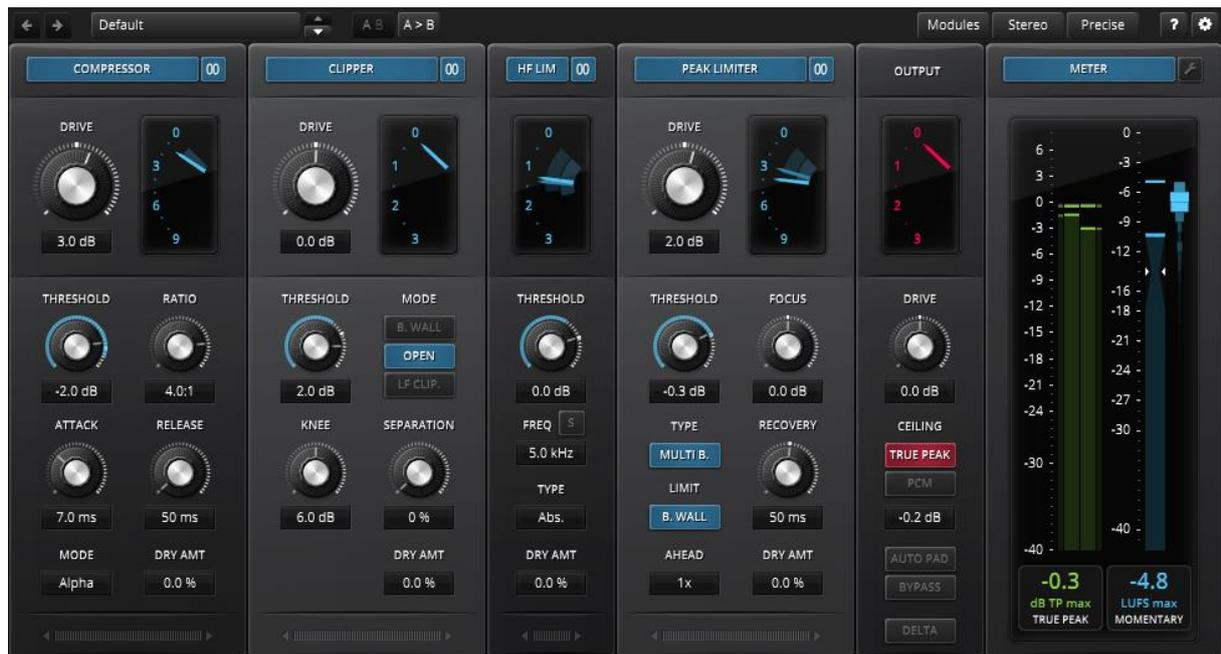
*TDR Limiter 6 GE* is a modern dynamics compression and limiting toolkit featuring six specialized modules that can be arranged in variable order. Together, they cover a remarkable range of applications from delicate loudness control, to brutal “brick-walling” and creative mix bus crunching.
