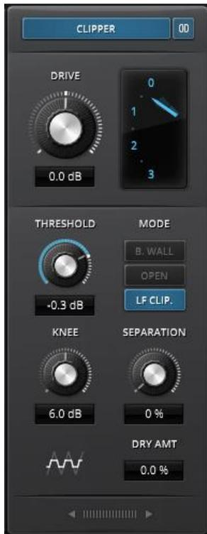
The clipper module is specifically meant to handle instant/short term dynamic events. The default mode offers a safe brick wall operation. Two further modes relax this strict behavior.
