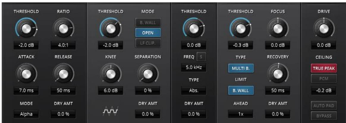
The next row, the "body", offers detailed access to every module's behavior. Note that every movable module also features its own **Threshold** (or **Range**) control, and a **Dry Mix** text box.
