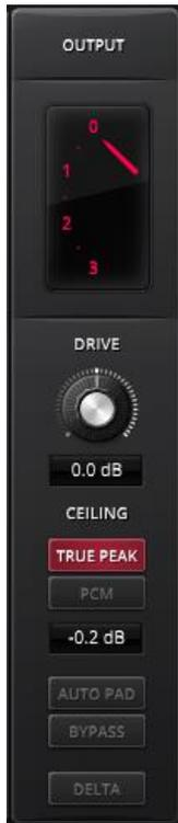
This output module provides a final means of controlling any remaining overshoots, thus guaranteeing that the output signal level doesn't exceed the value defined by the output ceiling text-slider.
