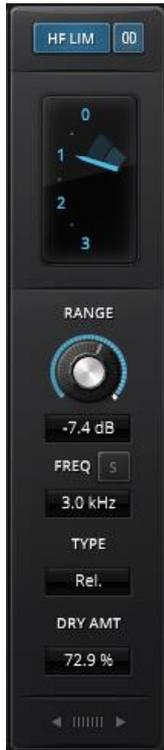
The High Frequency (HF) Limiter module's main task is the reduction or compression of excessive high frequency content.
