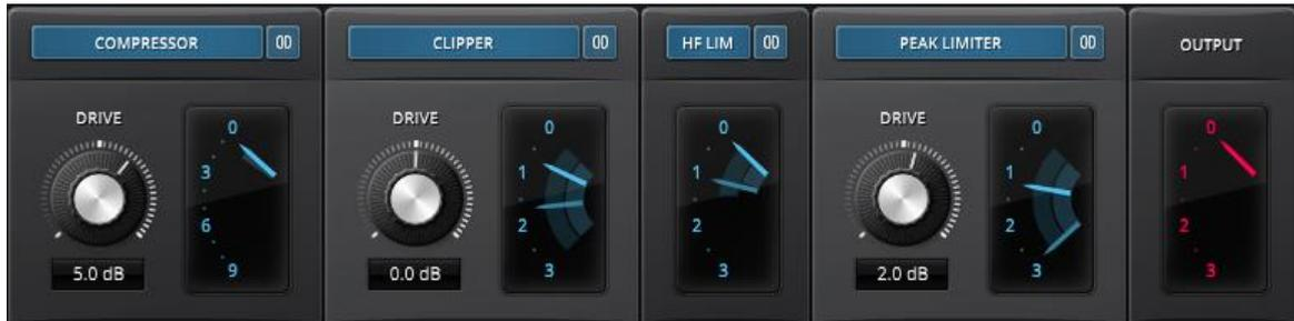
The upper row with big **Drive** knobs and VU style gain reduction meters contain the most important controls that you'll need to set up Limiter 6 for new material. On top of each module sits a local bypass button and a stereo/stereo + width switch. The big knobs drive the various modules and push them into gain reduction (see "Gain staging in Limiter 6" below for more details).
