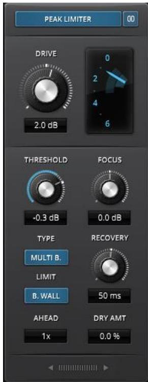
The peak limiter module is specifically meant to **control the extension of mid to short term dynamic events** without introducing excessive audible distortion.
