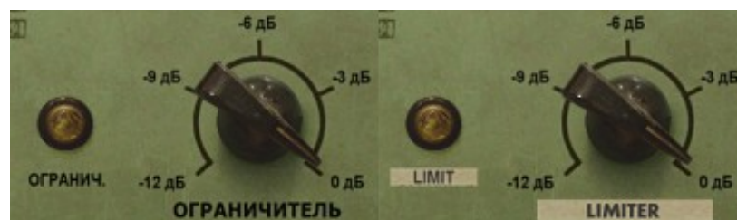
Pic 13. Limiter light indicator and control
