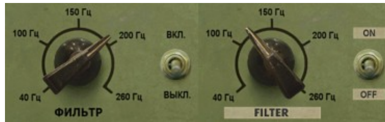
Pic 8. Side chain signal high-pass filter switch and control
