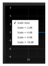
This ruler describes the extent of the main equalization curves (the frequency magnitude, width, and balance applied by the equalizer). The ruler will automatically adapt to fit the given curves into the visible area by default.
