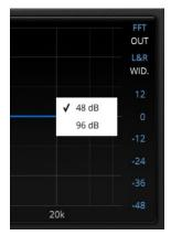
This ruler describes the extent of the analyzer curves (the signal's own frequency magnitude, width, and balance, depending on the selected mode).
