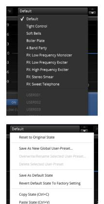
The preset dropdown list offers quick access to factory settings and user presets. Alternatively, the up/down buttons allow you to cycle through the presets. Note that some presets represent "flat" starting points, while others prefixed "FX:" demonstrate certain features and techniques.
